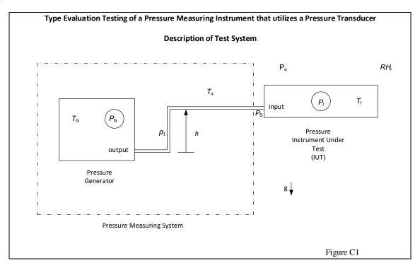
The instrument under test (IUT) is a pressure measuring instrument that utilizes a pressure transducer that, for the sake of illustration, will be considered to be configured in the so-called 'gage mode', meaning that one side of the transducer is open to ambient (atmospheric) pressure (denoted in Figure C1 by  $P_a$ ).
